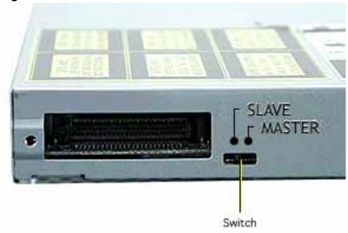
2. Install the connector board on the replacement optical drive, and secure it to the drive with the two screws. (Figure 13)
